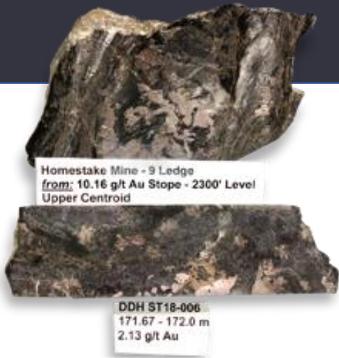
Standby DDH ST18-006 Core Sample (below) compared to Homestake 9 Ledge sample (above). Similar mineralization & alteration observed.
